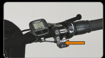
In its delivery state the scooter accelerates gently, making it very easy and safe to control. If you prefer acceleration to be very quick, you can increase the scooter's acceleration. With activated Turbo button (on 1) the acceleration is quick, with unactivated Turbo button (on 0) the acceleration is gently.
