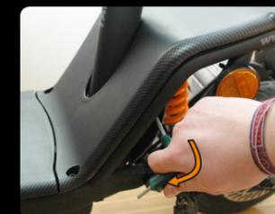
The scooter is delivered with one short and one long seat post. As delivered the seat is affixed to the long post. Select the seat post appropriate for your seat height and if required attach the seat and the reflector to the short seat post. Insert the desired seat post into the designated brackets on the scooter. Then screw it in tightly from the side.
