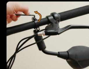
Remove the mirror from the small carton. Open the clamp with the included tool and then facing down on the left side affix the mirror to the part of the handlebar protected by a fiber band.
