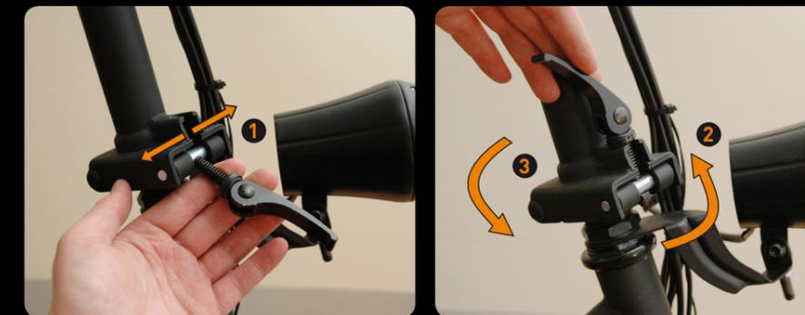
① Before folding upright push the bolt to the side and then fold the handlebar completely upright. Push the bolt back, ② fold the securing screw with the spring upright and ③ then fasten the hinge with the black safety clasp.
