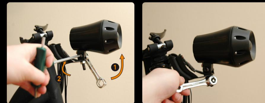
① Align the front light in the direction of travel and ② screw it in tightly on the side using the wrench and the T Allen wrench. **Make sure not to bend the light bracket!**
