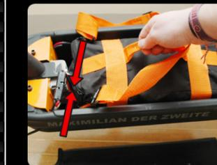
Take the battery out of the small carton and, if necessary, remove the transport retaining band from the plug. Use the ignition key to open the battery compartment and insert the battery. Then connect the plugs, which for reasons of safety will require a bit of effort to connect
