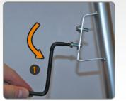
Remove the basket from the small carton and screw it to the mount on the seat tube.
