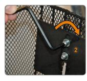
2 Place the basket on the mount, push the screws through the slot and fasten them to the mount. For safety reasons, the basket is elastic. Should it be deformed, push it back into shape with your hands.
