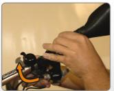
Remove the screw nut and the washer from the rear-view mirror.
