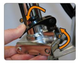
1 Before folding upright push the bolt to the side and then fold the handlebar completely upright. Push the bolt back, 2 fold the securing screw with the spring upright 3 and then fasten the hinge with the black safety clasp.
